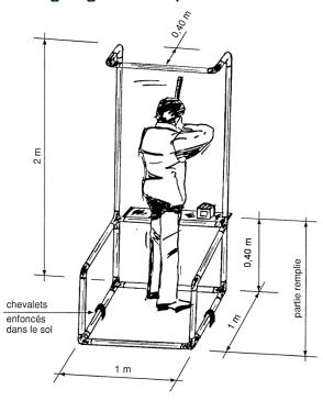
Shooting station made of coloured PVC tubing, [] 50 mm
